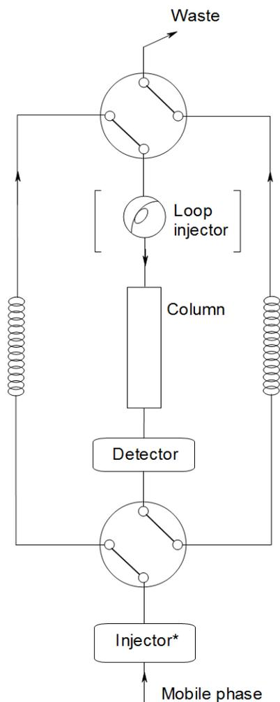
***Use of alternating loops for recycling in analytical liquid chromatography***
