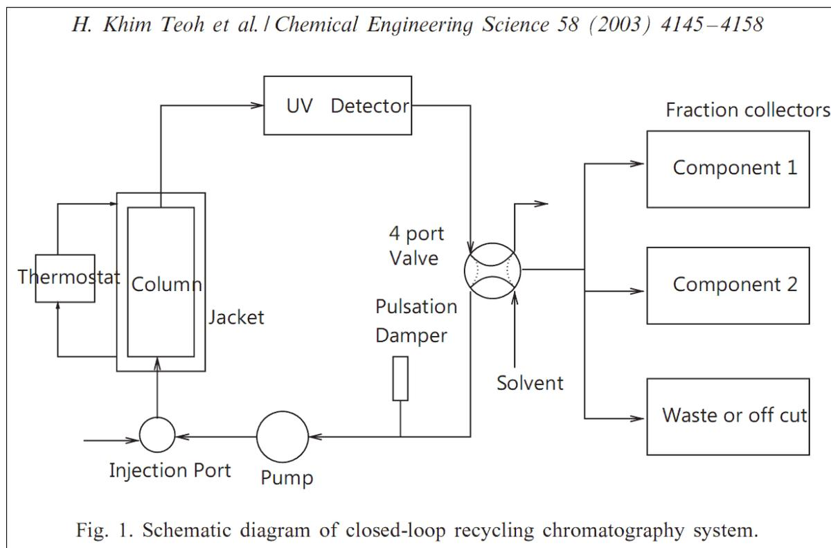
***Recycling through the pump in preparative liquid chromatography. For column switching two systems are used in tandem.***
