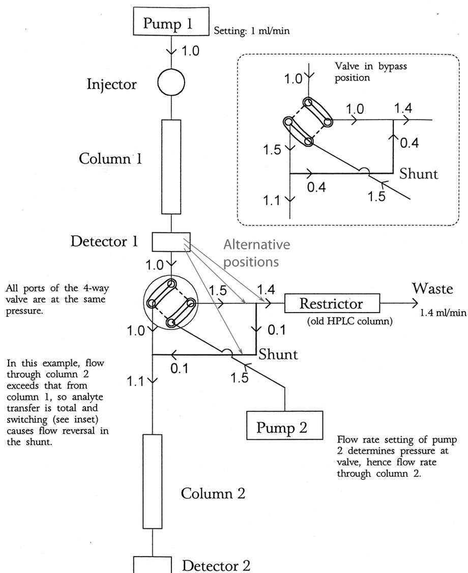
***Pressure balancing with total transfer to the second column.***
